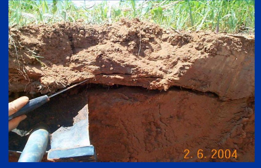
Compacted, platy replaced topsoil over highly compacted tails/slimes subsoil.
