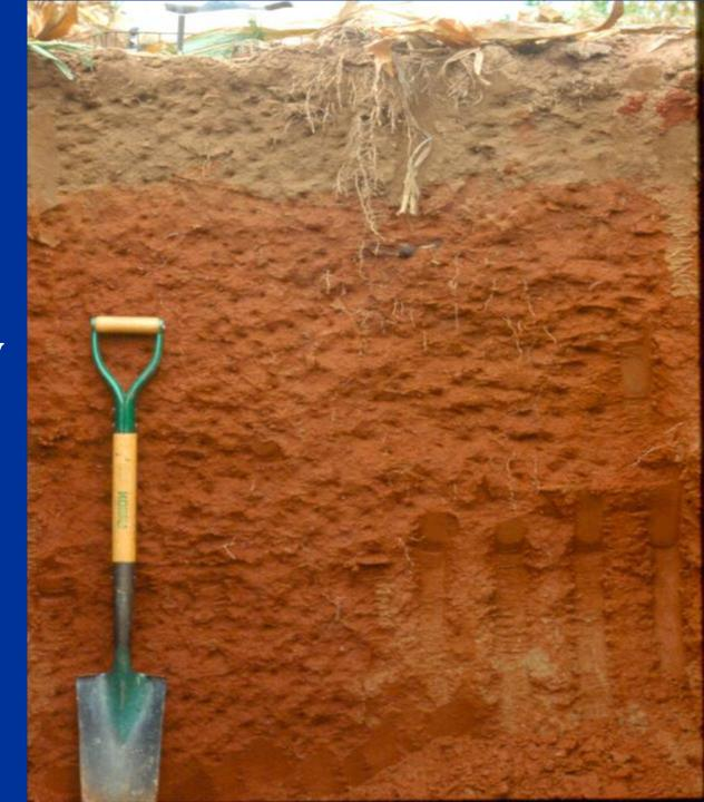
Test pit filled with mixed slimes/tailings from pilot plant in April, 1995.
